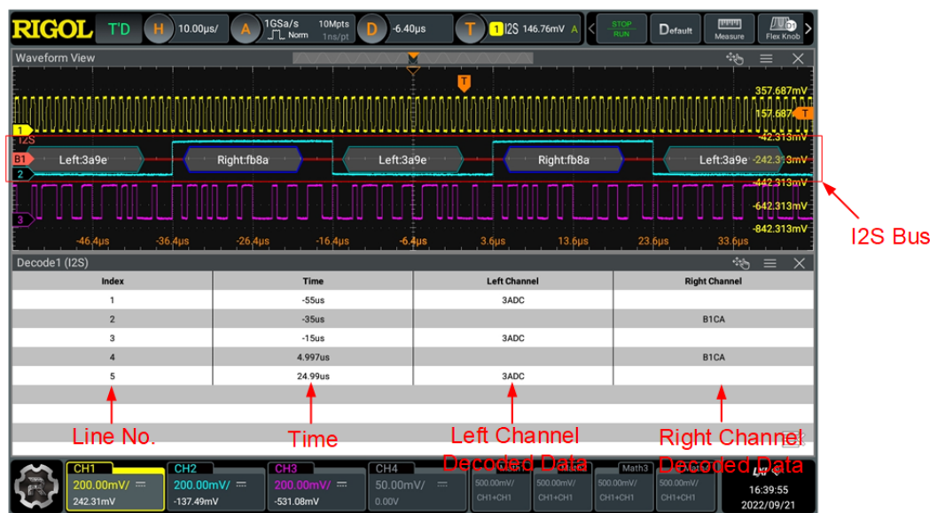
Figure 15.19 I2S Decoding Event Table
