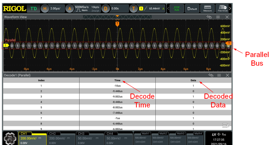
Figure 15.3 Parallel Decoding Event Table
