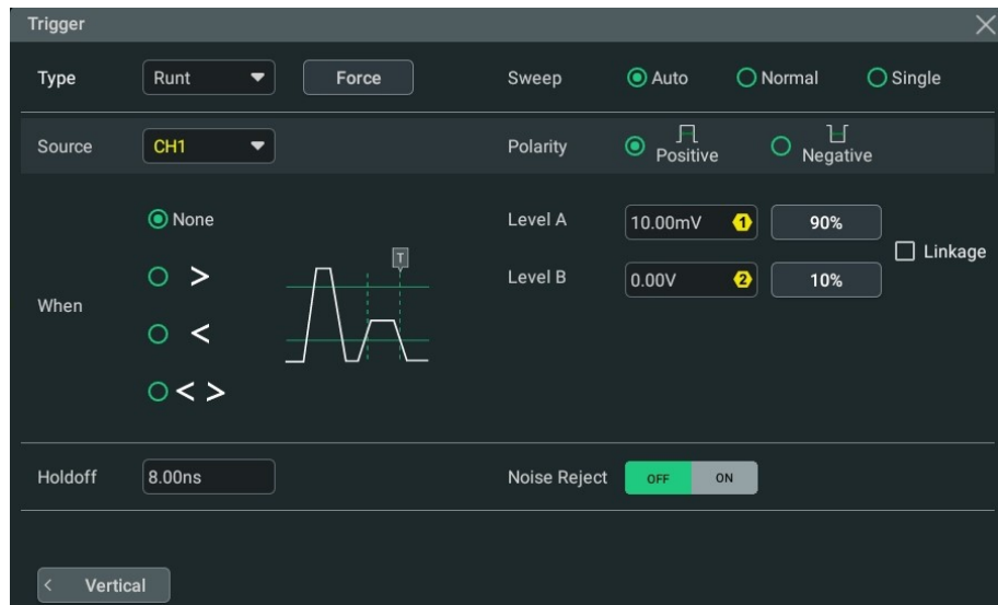
Figure 8.16 Runt Trigger Setting Menu
