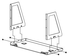
(2). Install the front plate: fix the front plate onto the side plates (left and right) of the rack using six M4 screws.
