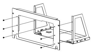
(3). Place the instrument: place the instrument by aligning it with the edges of the side plates (left and right) and front plate of the rack and fix the instrument onto the bottom plate through presser feet using four M4 screws.
