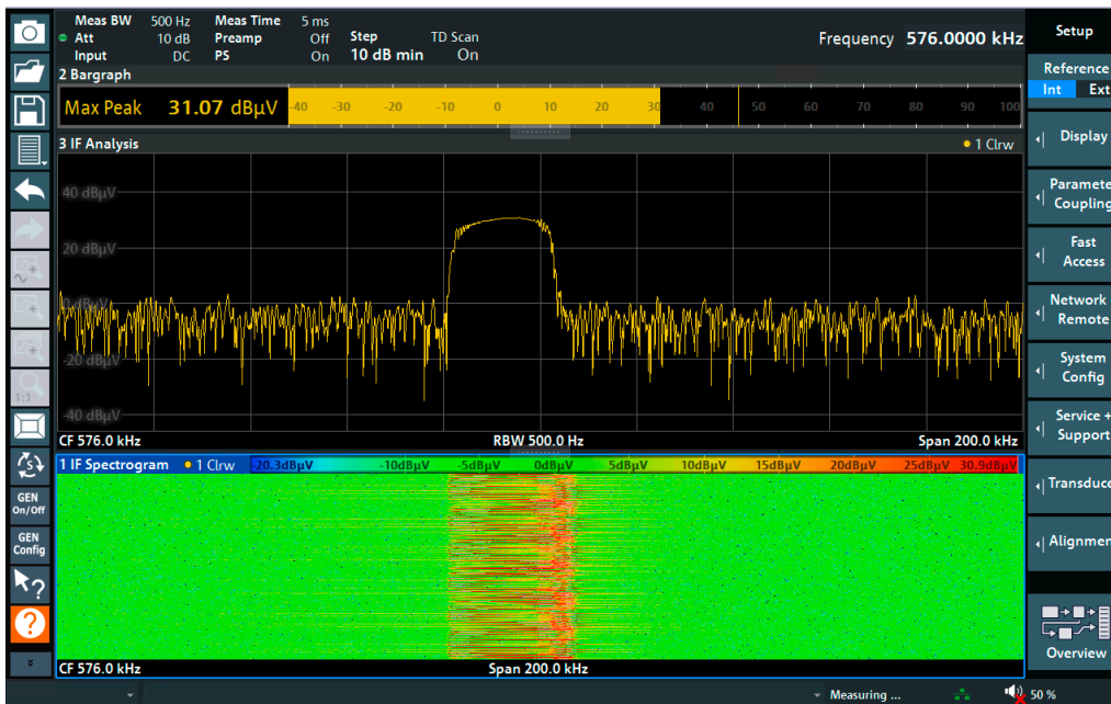
Analysis of the emissions of a LED lamp at 576 kHz using bargraph display in combination with IF spectrum and spectrogram function. The dynamic behavior of the signal, especially in the range of 560 kHz to 585 kHz, is clearly visible.
