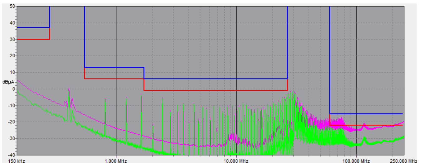
Figure 19: measurement result using an automotive manufacturer standard with tougher limits compared to CISPR25 Class5; peak detector (green) and quasi peak detector (pink); measured in 5 cm distance from DUT on positive and negative supply line; set up in shielded tent
