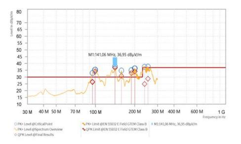
Again QP limits and a peak detector measurement. Now, several spurious cross the QP limits and as QP detector amplitudes are always lower than peak detector amplitudes, there is a chance that the spurious are still below the QP limit line. Consequently, at the frequencies with the highest spurious levels, QP
