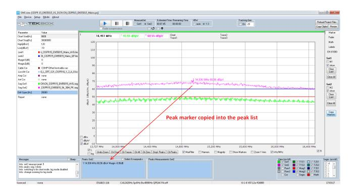
Finally, a QP measurement is carried out, selecting the peak in the peaks list, right mouse button and selecting Measure (consider drift). After the measurement, the QP measurement result appears in the graph window and peak measurement list. The result is at the same frequency, which shows that the spurious maximum has not drifted.
