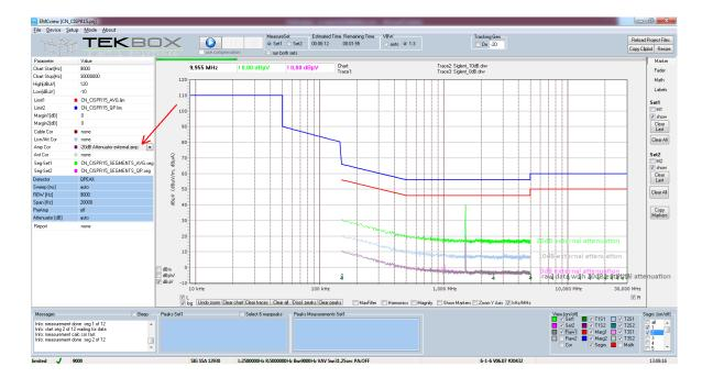
And here the zoomed view. The amplitude values (raw values) obtained from the analyzer are not compensated with respect to the internal attenuation. EMCview compensates the raw values based on the content of the amplitude file.
