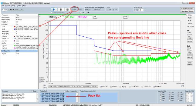
The peaks are displayed in the graph, using marker circles; furthermore the frequencies, amplitudes and offset to the limit line are displayed in the peak list.
