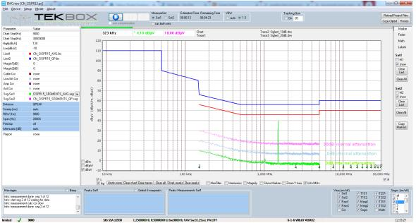
And here the zoomed view. The amplitude values obtained from the analyzer are already compensated with respect to the internal attenuation.
