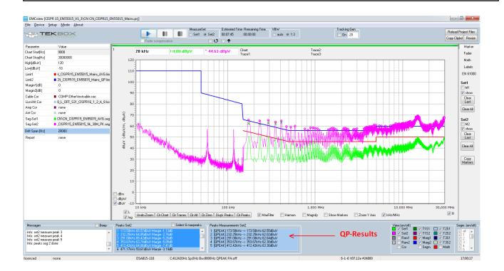
The QP Levels are furthermore displayed in the graph, as can be seen in the zoomed graph of the screenshot below. As expected, the QP results are always in between the levels of the peak and average measurement. The QP re-measurement shows that the first two spurious would pass QP limits with some tiny margin.
