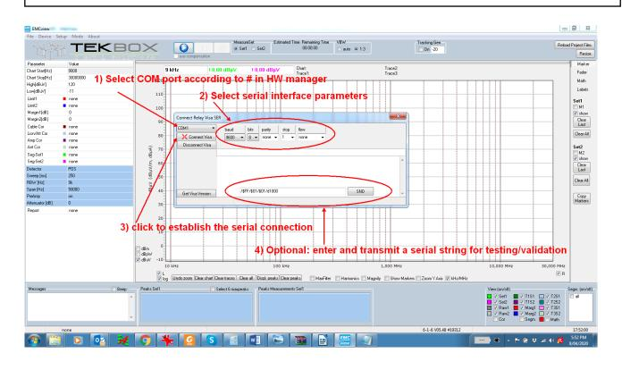
In order to automatically transmit test strings, they need to be entered into the desired segment file. You can add two serial command strings to each segment. Command SCPI\_A will be executed before the sweep of the corresponding segment. Command SCPI\_B will be executed after the sweep of the corresponding segment.
