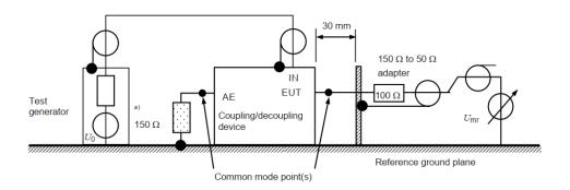
Voltage division factor RF-port to EUT-port: 150 kHz – 80 MHz: 9.5 dB ± 1dB
