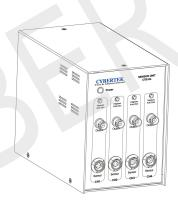
CTB104 sensor unit: the sensor unit for the probe. 4 channels for 4 current probes at same time, including probe connector, BNC output port, degaussing button and power supply indicator.
