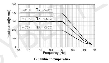
CTB500A Current rated value vs. Frequency curve
