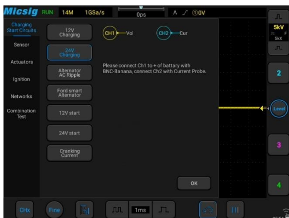
▲ Support 12/24V Charging & Start circuit, AC Ripple, Cranking Current tests
