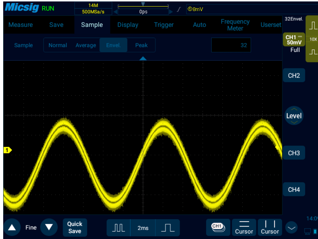
Figure 11-8 AM Signal in Envelope Sampling Mode (32)
