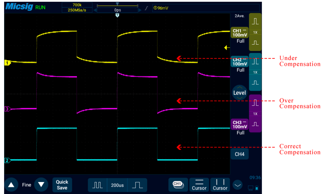
Figure 2-14 Probe Compensation
