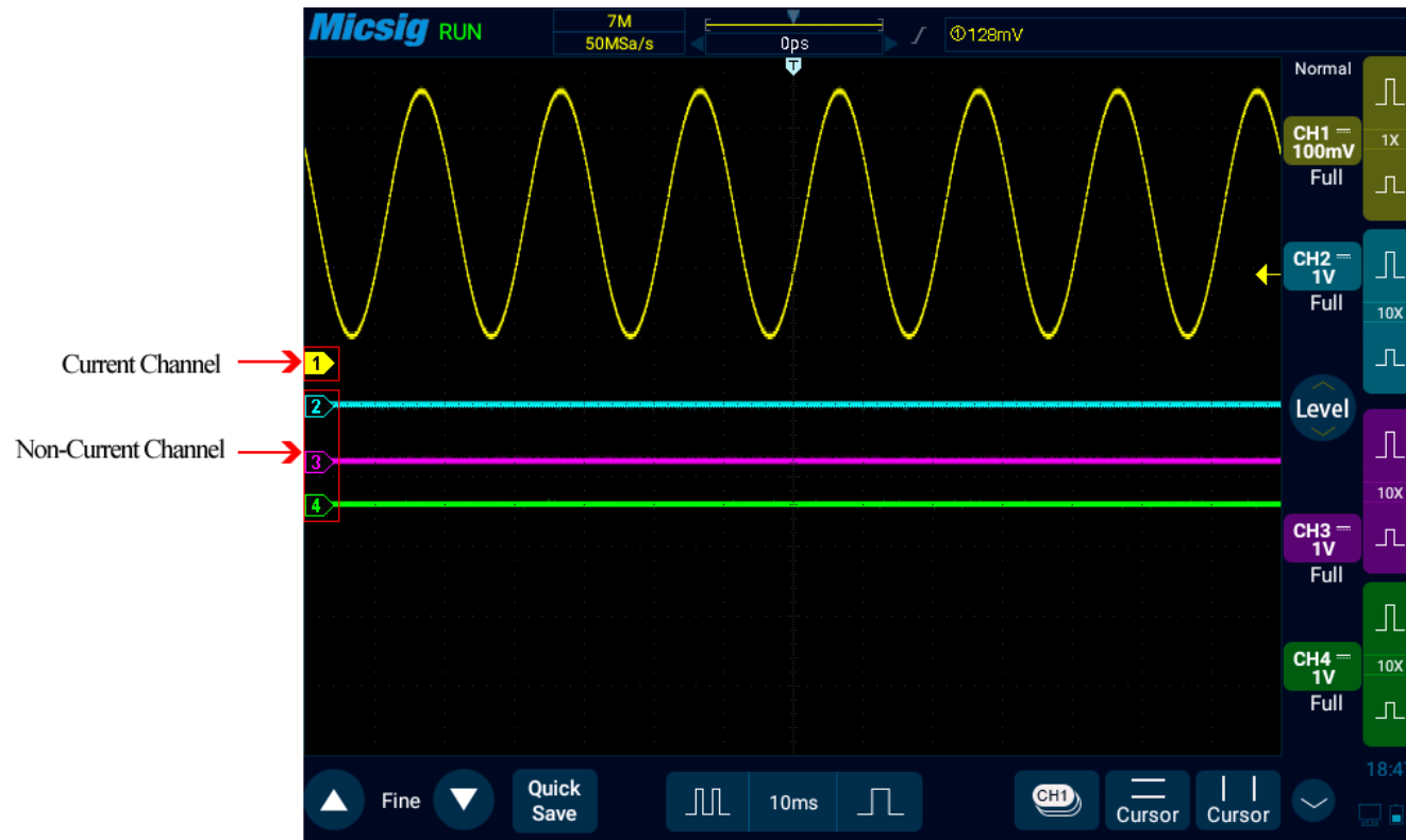
Figure 5-2 Current Channel and Non-Current Channel
