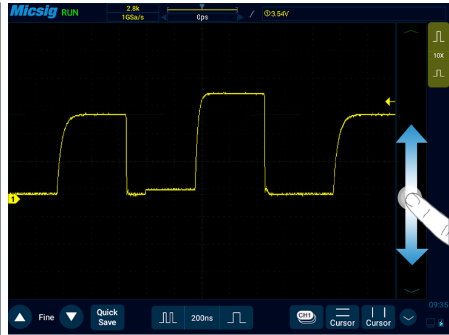
Figure 6-4 Abnormal Signal Captured by Setting Trigger Level
