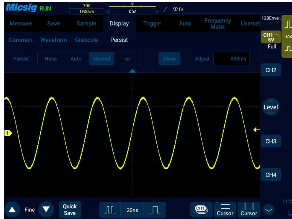
Figure 10-4 20MHz Sine Wave Variable Persist 500ms
