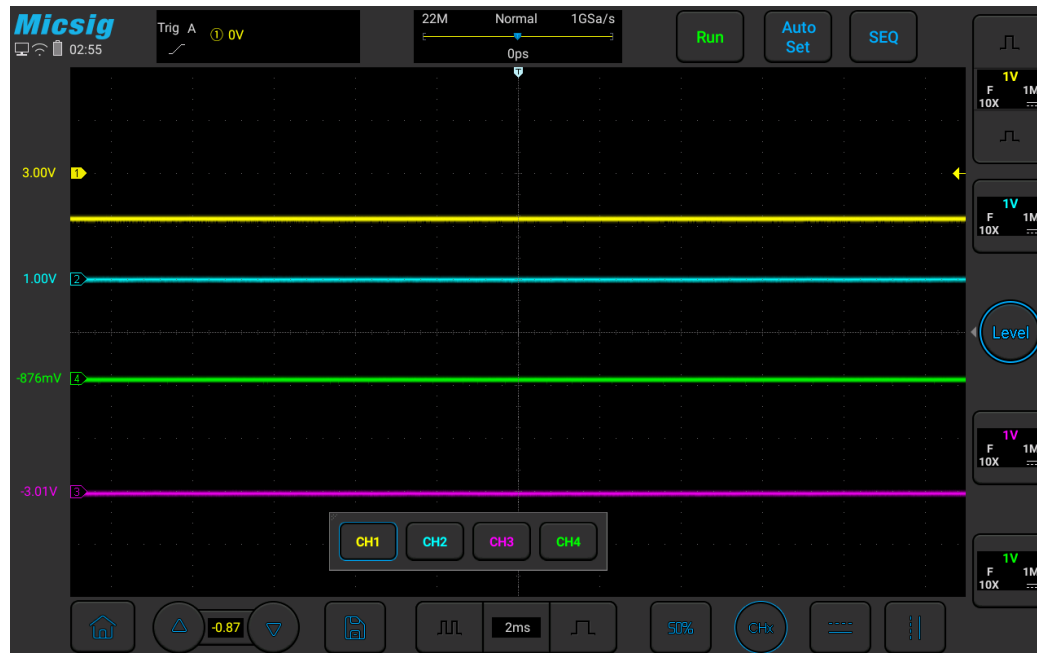
Figure 2-13 Manual zero calibration
