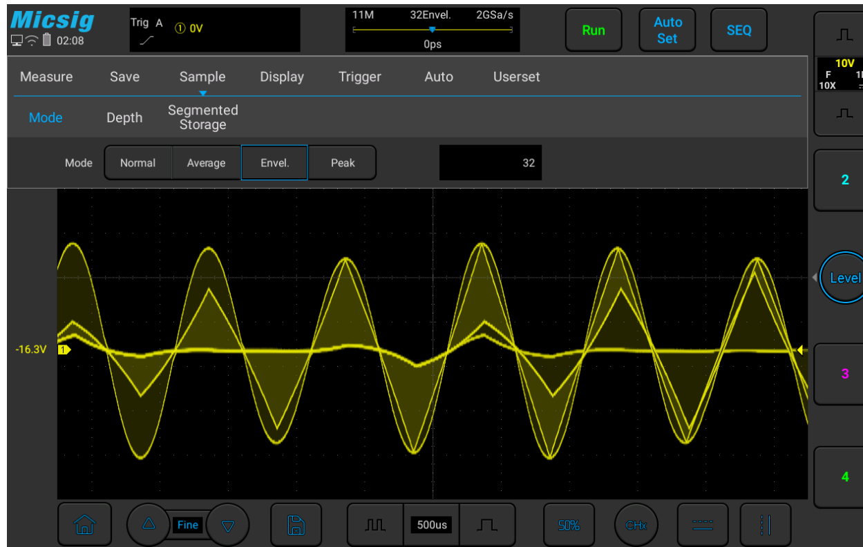
Figure 10-8 AM Signal in Envelope Sampling Mode (32)
