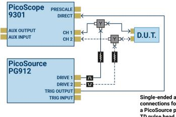
Single-ended and differential connections for TDR testing, using a PicoSource pulse generator with TD pulse head outputs
