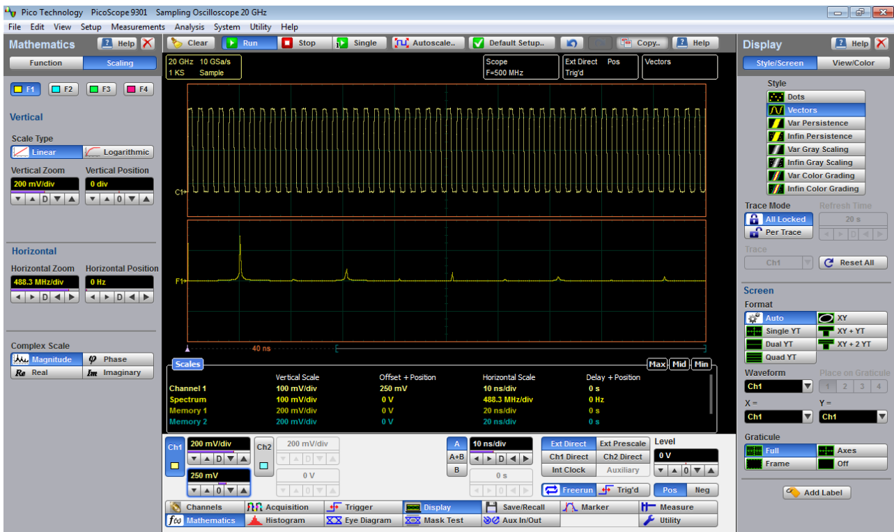
Spectrum Magnitude of 500 MHz pulse waveform
