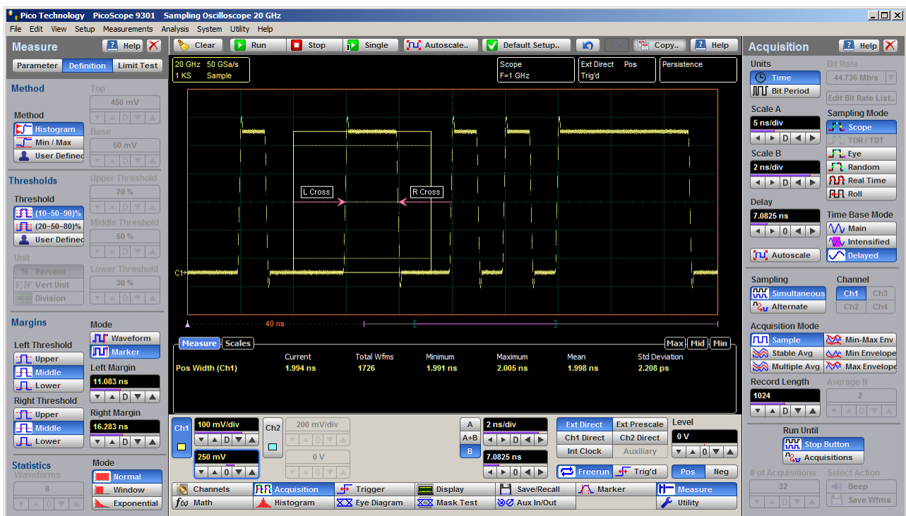
Correct position of both margins provides width measurement of second short pulse
