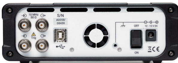
Figure 3 - Rear panel of the AS108
