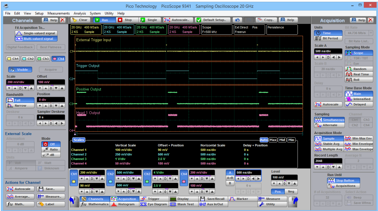
Timing diagram for external triggered mode (2 μs period of external signal)
