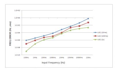
The graph doesn't include the effects of trigger error. To place an upper bound on the added effect of this error term, it's necessary to determine the frequency error from the proper graph and add a trigger error term as the following equation:
